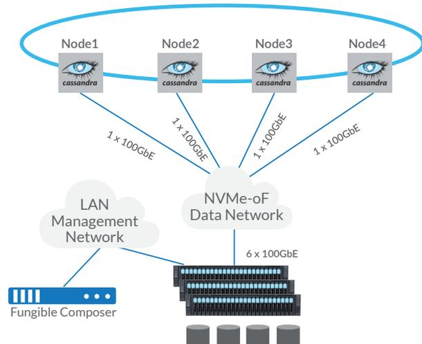
Figure 2. Apache Cassandra Deployment Using Fungible Storage Cluster Disaggregated Storage
