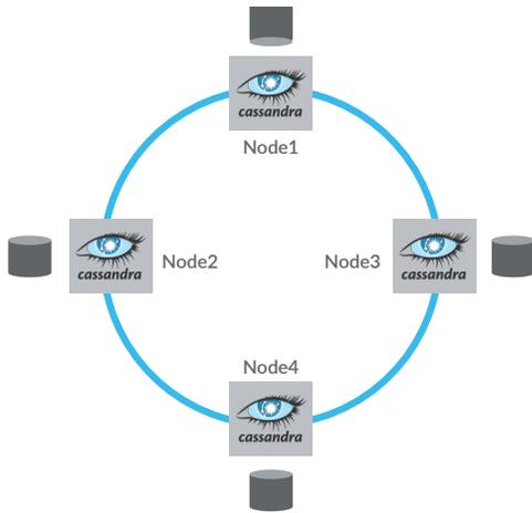
Figure 1. Traditional Apache Cassandra Deployment Utilizing Direct-Attached Storage (DAS)
