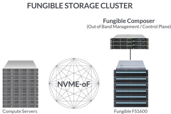
The Fungible Composer operates on a control plane that is distinct from the FS1600s' storage data plane. It runs on a 3-node self-contained quorum-based cluster for scalability and high availability. Such separation of control and data plane allows for linear scalability in capacity and performance on FSC.
